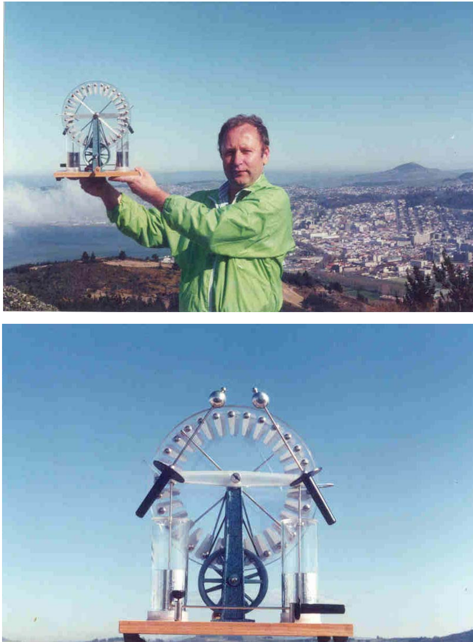
Fig. 11. The appearance of the Wimshurst electrostatic machine, model V5-43, produced by the Polish factory named "Fabryka Pomocy Naukowych w Nysie" (address: ul. Slowianska 43, 48-300 Nysa, Poland). It works very effectively and is an excellent illustration of the principles involved in the generation of electrostatic charges. The majority of Polish schools currently utilize this machine for conducting electrostatic experiments, e.g. for demonstration and experimenting with electric sparks. The comparison of the machine with the author who holds it, gives an idea about its size (on the second plan the New Zealand city Dunedin is visible). The device shown here has two plexiglas disks of the diameter 250 mm. Each of these disks contains 30 electrodes. The disks rotate on bronze bearings, and are hand-propelled with two pulleys linked to a winch via two elastic belts. In 1991 this machine purchased and collected directly from the factory costed an equivalent to around 30 dollars USA (this amount did not included any delivery/postage costs). The above machine is highly recommended as a starting point for people initiating their own research on telekinetic powerstations. It can easily be converted into an interim electrostatic device in subsection 5.6. described under the name "Dr Pająk's model", which can later be converted into a telekinetic influenzmaschine.
