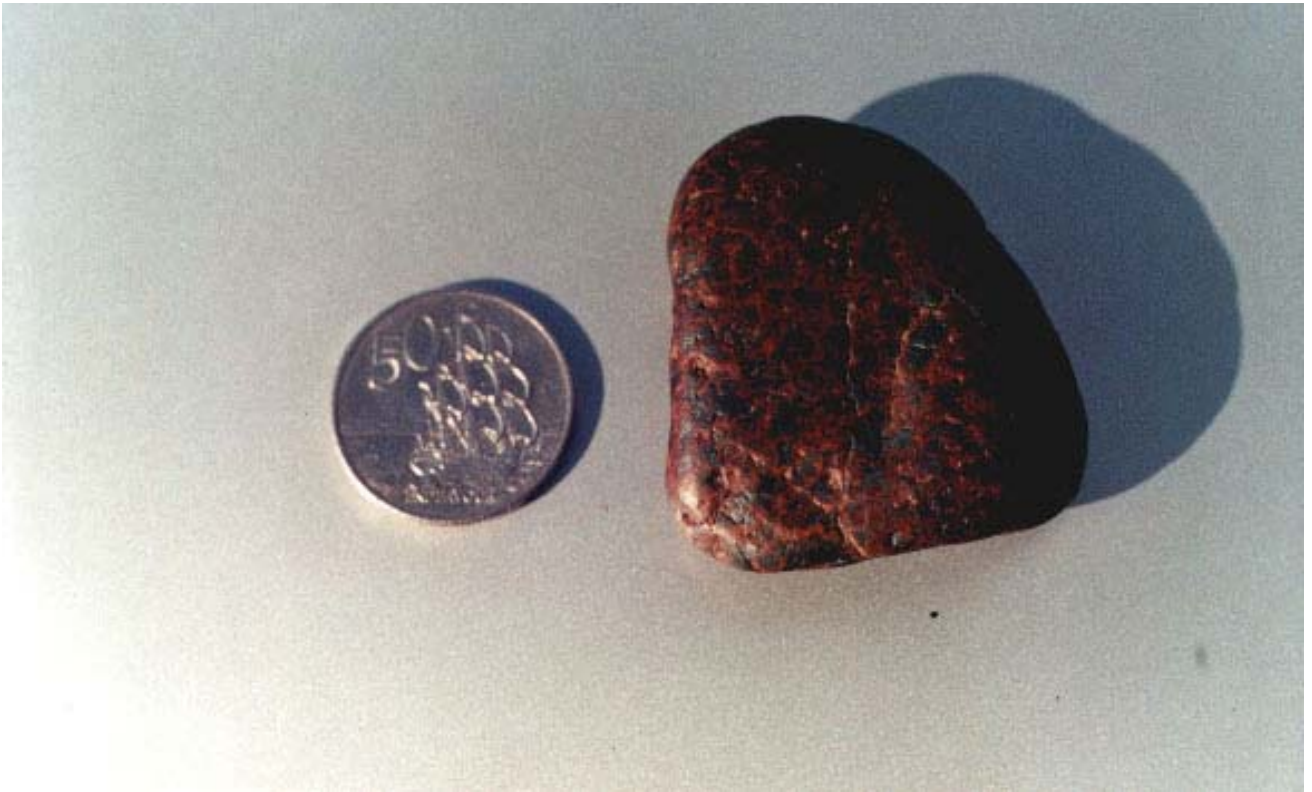
Fig. C14. A magnetized metallic piece found in the vicinity of the Tapanui Crater. To reflect its dimensions, a coin of 31 mm in diameter is also photographed. The analysis revealed that this piece contains around 60% of silicone, 30% of iron, and 10% of aluminium. (It is worth mentioning that in its pure form aluminium does not appear in nature.) Taking into account the melted surface, aerodynamic shape, compressed structure, turbulent magnetization, and unusual composition of this piece, it can be concluded that it most probably originates from parts of a spaceship which were mixed with local soil, compressed, smoothed on the surface, and magnetized during this explosion. It should be stressed that four chunks of such material were found so-far. Except for the one presented above from the author's collection, another piece is held by Mr Ken Goldfinch (26 Lothian Street, Maori Hill, Dunedin). Two further gold-coloured magnetized pieces that look like they have been cut out from a piece of medical instrument are at the disposal of the Geology Department at Otago University, Dunedin, New Zealand.
